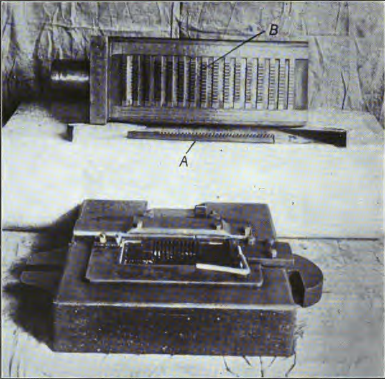
FIG. 83.—Rack-cutting broach and fixture.
